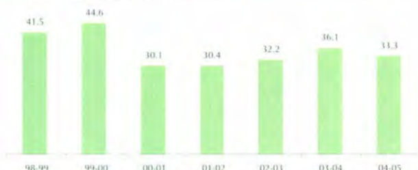
Specific Energy Consumption in the Bhadrachalam Paperboards Mill (Giga Joules/tonne of paperboard)
