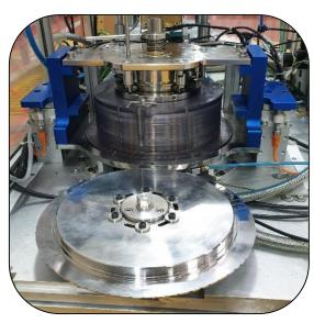
In-house developed sub-assembly for double-capsule filter manufacturing
